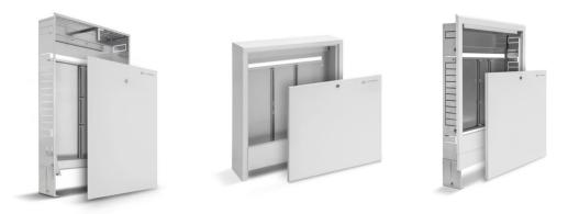
The design of the cabinets for surface heating/cooling applications allows the installation of manifolds with and without a mixing system. The cabinets also provide space for automation controls system devices (e.g. terminal blocks). They can be fixed onto special rail using a screws or by hooking onto a standard DIN rail. Both rails, depending on the type of installation cabinet, are located in the upper part of their construction.
