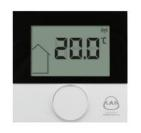
Wireless room thermostat with LCD is a device, which controls the KAN-therm Smart electrical terminal block (24 V or 230 V) via radio waves. It is used to record the temperature in a room and to set desired temperature, in a heating zone assign to it.
