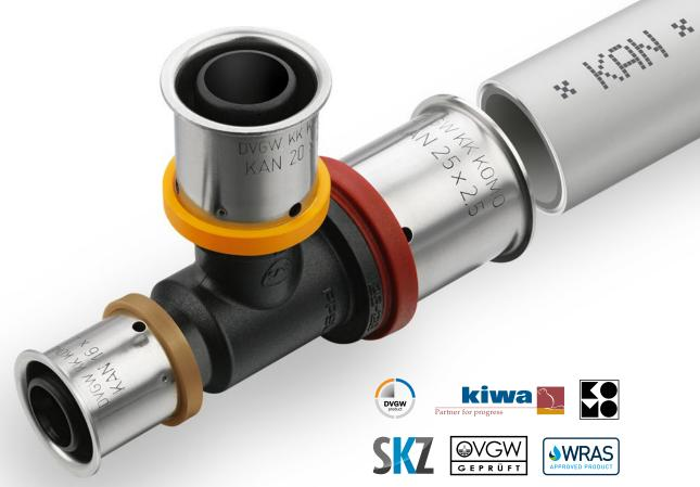
SYSTEM KAN-therm Press is a modern, complete installation system consisting of composite polyethylene pipes with aluminum layer and plastic PPSU or brass fittings with a diameter range between 16 and 63 mm.
